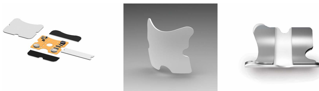
Figure 1. Device description. Left: Exploded view depicting the main components; Center: Front view; Right: Skin-side view.
