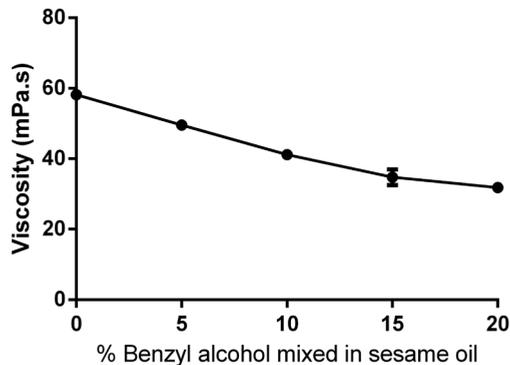
Figure 3.3: Viscosity of different concentrations benzyl alcohol mixed with sesame oil. No other substances were added. Results expressed as mean and standard error of the mean ( $n=3$ ), unless standard error is smaller than the symbol.
