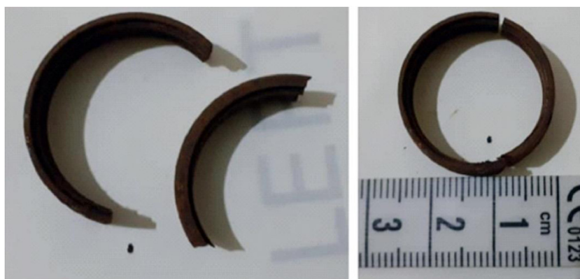
Fig. 3. Showing the ring piece after it was cut and reassembled to estimate diameter.
