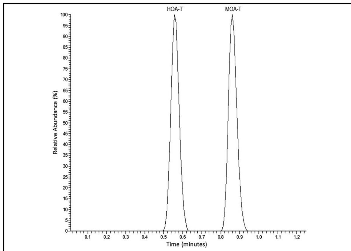
**Fig. 2.** Representative chromatogram of HOA-T and MOA-T. HOA-T, hydroxylamine derivative of testosterone; MOA-T, methoxyamine derivative of testosterone.
