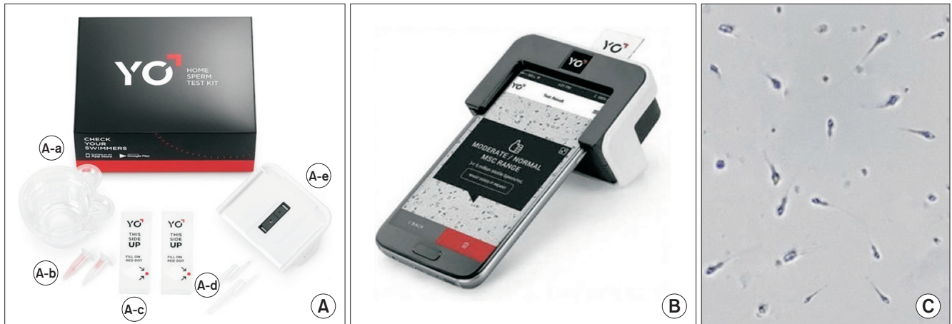
Fig. 5. The YO Home Sperm test device and components. (A) YO kit contents, including, (A-a) collection cup, (A-b) liquefaction powder, (A-c) fixed coverslip slide (d) fixed volume transfer pipettes, and (A-e) YO testing clip. (B) The assembled YO clip with inserted testing slide. (C) Sample as seen on the phone screen.
